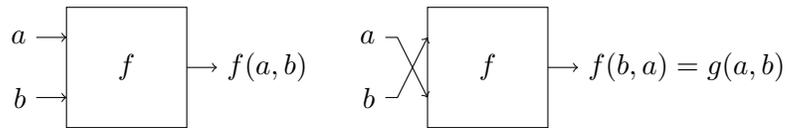
**Figure 14.25:** A switching function of two variables
