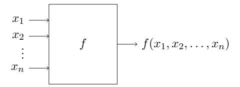
Figure 14.24 A switching function of n variables
